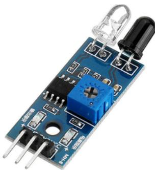
**IR Sensor (Infrared Sensor):** An IR sensor detects infrared light, allowing it to sense the presence or motion of objects. It's commonly used for proximity sensing or object detection in robots.
